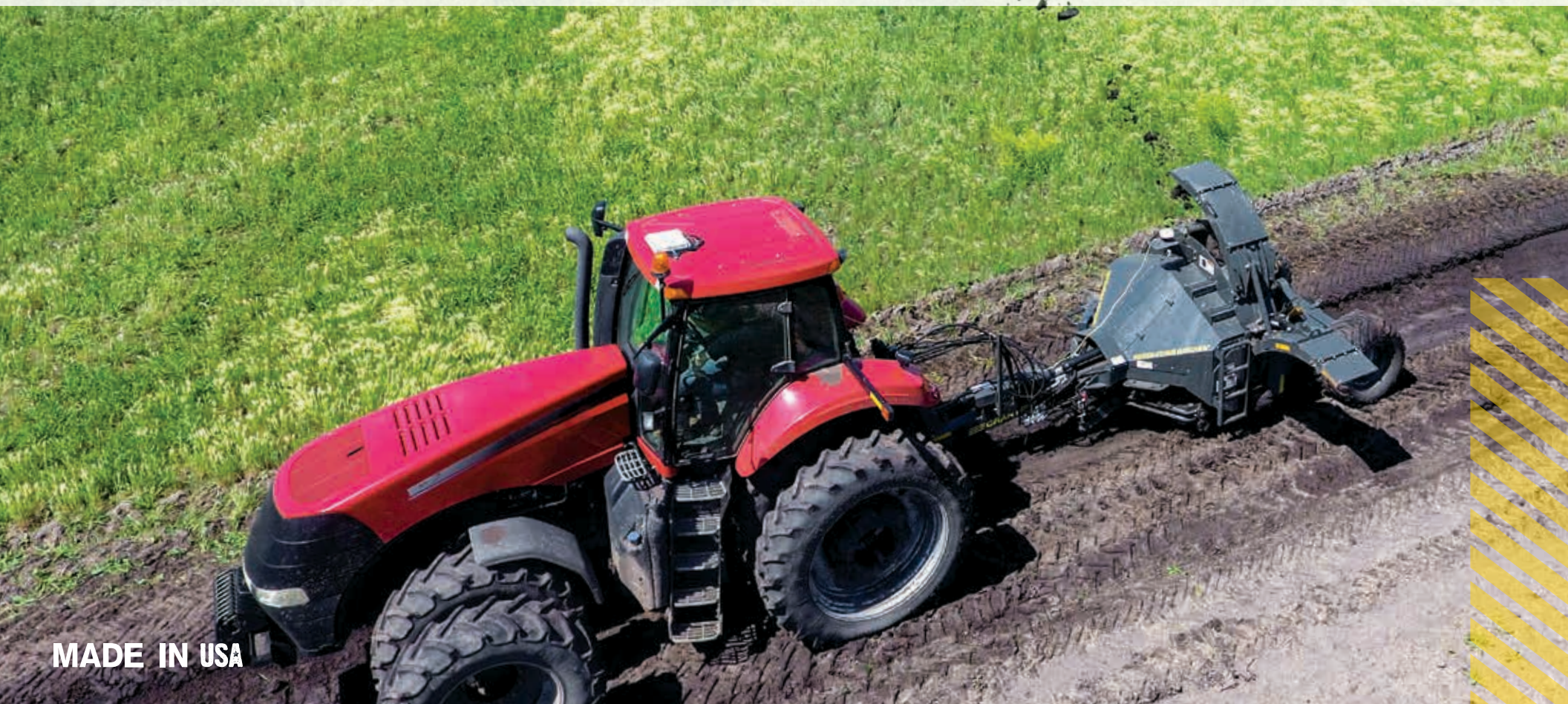
CROSS AUGER breaks up material for optimum performance, allowing up, down, fore, and aft adjustments.
